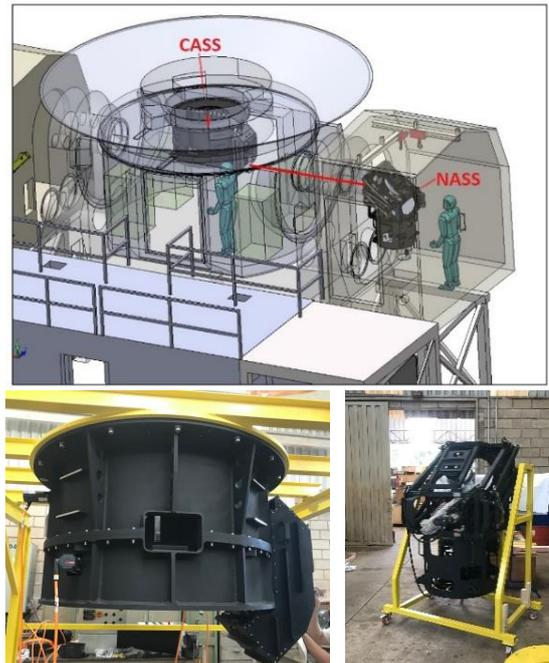
*Top: Overview of the NACOS mechanical design. Bottom: NASS and CASS, components of NACOS, in the process of integration and optical alignment in the premises of ALFA Engenharia (Araraquara, Brazil).*
