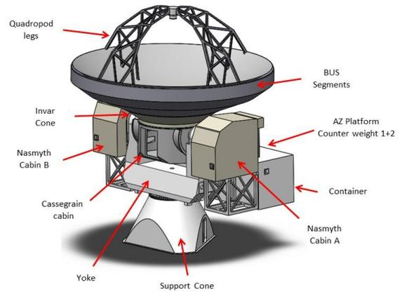
*Overview of LLAMA's antenna with an indication of some of its main components.*
